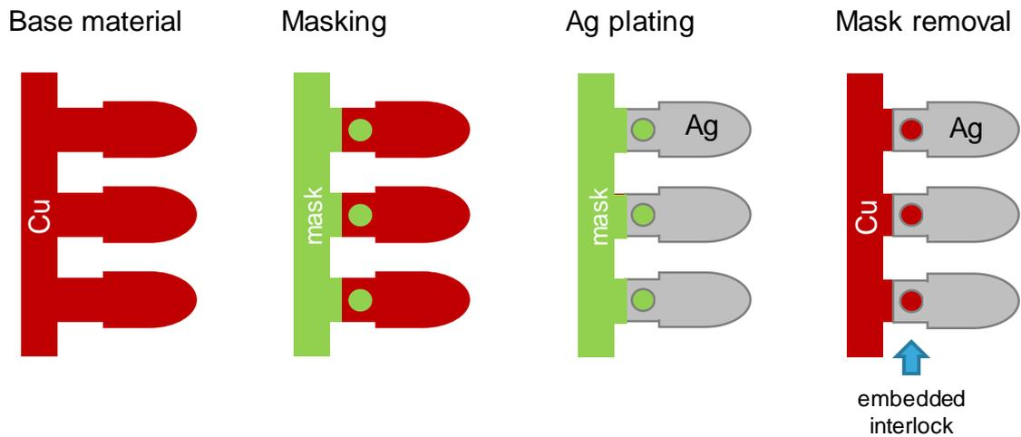
Fig. 4. Embedded interlock process flow.
