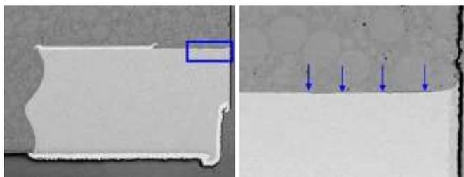
Fig. 1. Delamination along the EMC-to-carrier interface.
