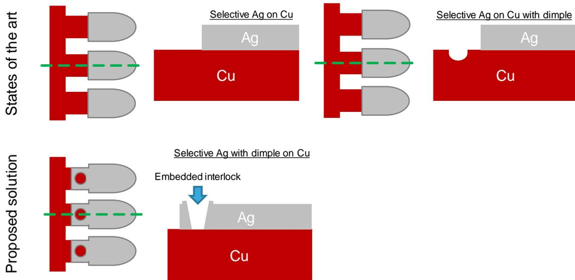
Fig. 3. Schematic representation of selective Ag on Cu, Selective Ag on Cu with dimple and the selective Ag with dimple on Cu.
