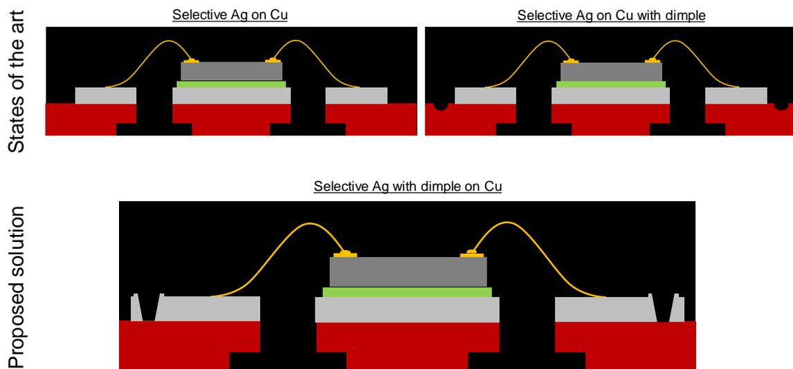
Fig. 5. Package cross-sectional construction using selective Ag on Cu, Selective Ag on Cu with dimple and the selective Ag with dimple on Cu.
