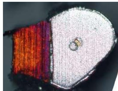
Fig. 2. Oxidized exposed copper (left) and Ag plated surface (right).
