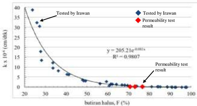
Fig. 6. The results of permeability test in the graph proposed by Irawan
