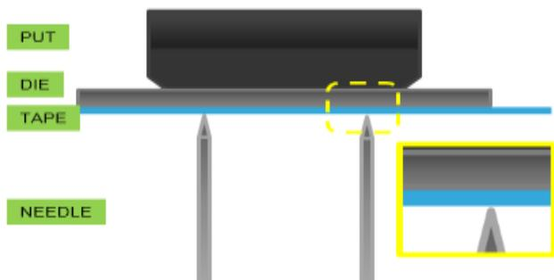
Fig. 2. Position of needle on standard packages.
