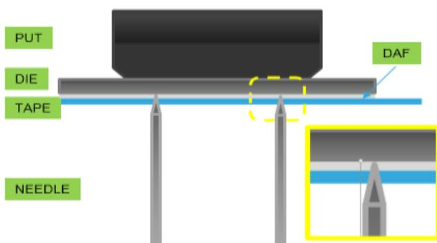
Fig. 3. Position of needle with DAF packages.
