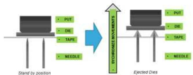
Fig. 1. Bond head movement during die attach process.
