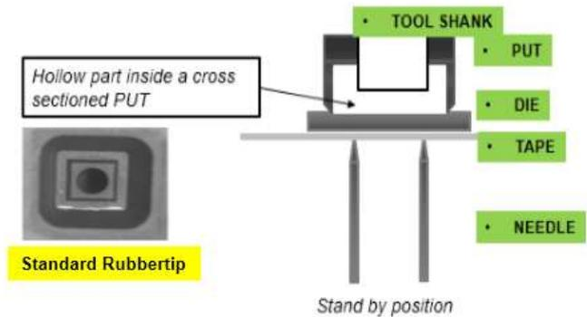
Fig. 4. Cross section of pick-up tool used on standard pick and place.
