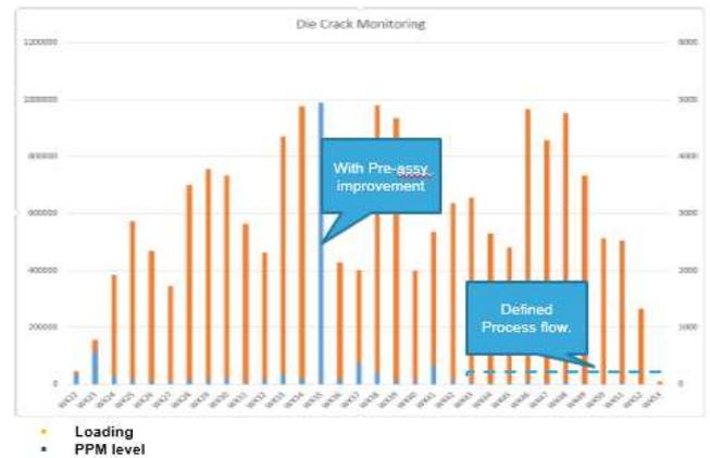
Fig. 9. Die crack trend, ppm level (blue) vs loading (orange).
