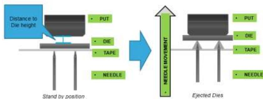
Fig. 8. Pick-up sequence with addition of distance to die.
