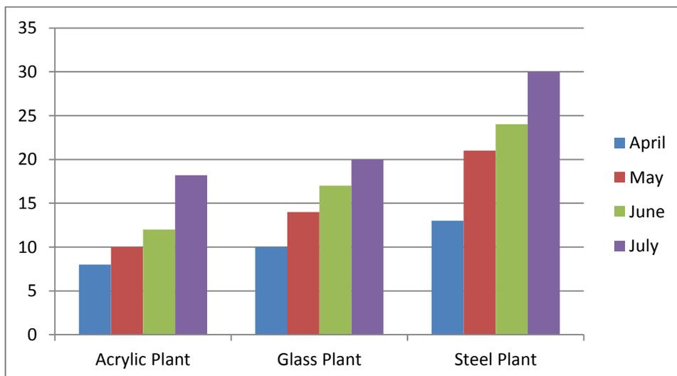
Fig. 5. Different desalinated Flow Rates in l/h for the three tested plants
