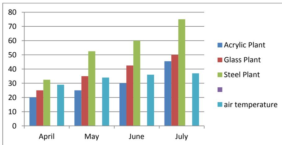
Fig. 7. Air Temperature (°C) and the Recovery Ratio (%) For The Three Applied Plants
