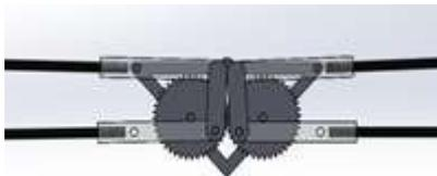
Fig. 6. Crank gear linkage mechanism
