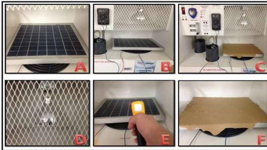
Fig. 1. The used apparatus in the tests: (a) the used PV, (b) the PV location, (c) the PV placed and covered entirely with the paper boards, (d) the light bulb, (e) the laser-IR-temperature gun in the process, (f) the paperboard covering the PV.
