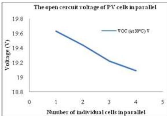
Fig. 7. The open circuit voltage of PV cells in Parallel (Individual Cells).
