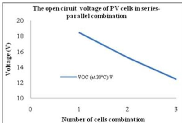
Fig. 8. The open circuit voltage of PV cells in series-parallel combination.
