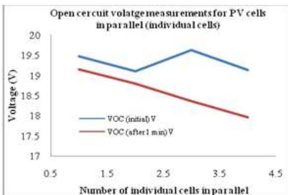
Fig. 4. Open circuit voltage measurements for PV cells in parallel (individual cells).
