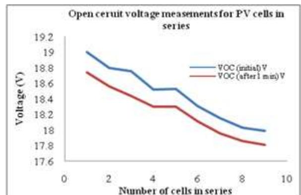
Fig. 2. The open circuit voltage measurement for the PV cells in series.
