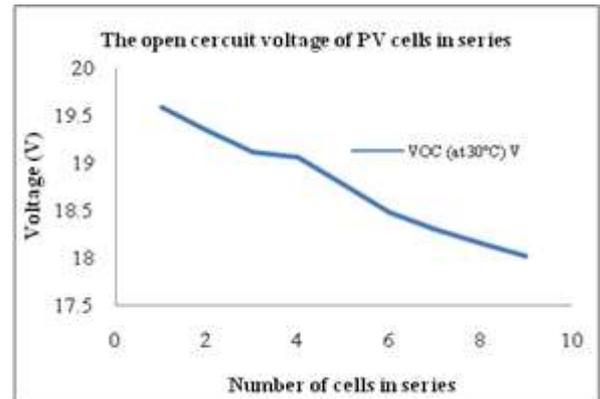
Fig. 5. The open circuit voltage of PV cells in series.
