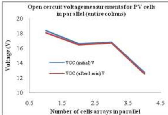
Fig. 3. Open circuit voltage measurements for PV cells in parallel (entire columns).
