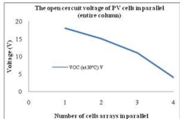
Fig. 6. The open circuit voltage of PV cells in parallel (entire column).
