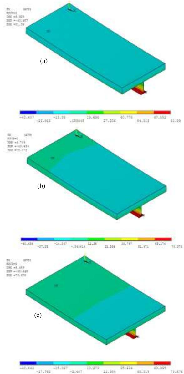
Fig. 7. Contour plots for the longitudinal stress for composite beam with different slab breadth, (a)  $b/L = 0.222$ , (b)  $b/L = 0.272$ , (c)  $b/L = 0.364$ .
