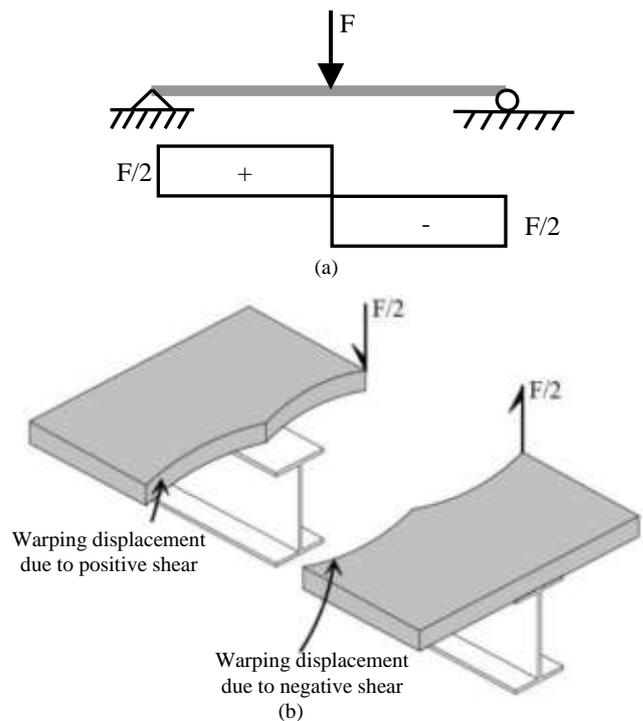
Fig. 3. Incompatible warping displacements at a shear discontinuity, (a) beam and shear force diagram, (b) warping displacement calculated from conventional theory (Oehlers and Bradford, 1999) [7].
