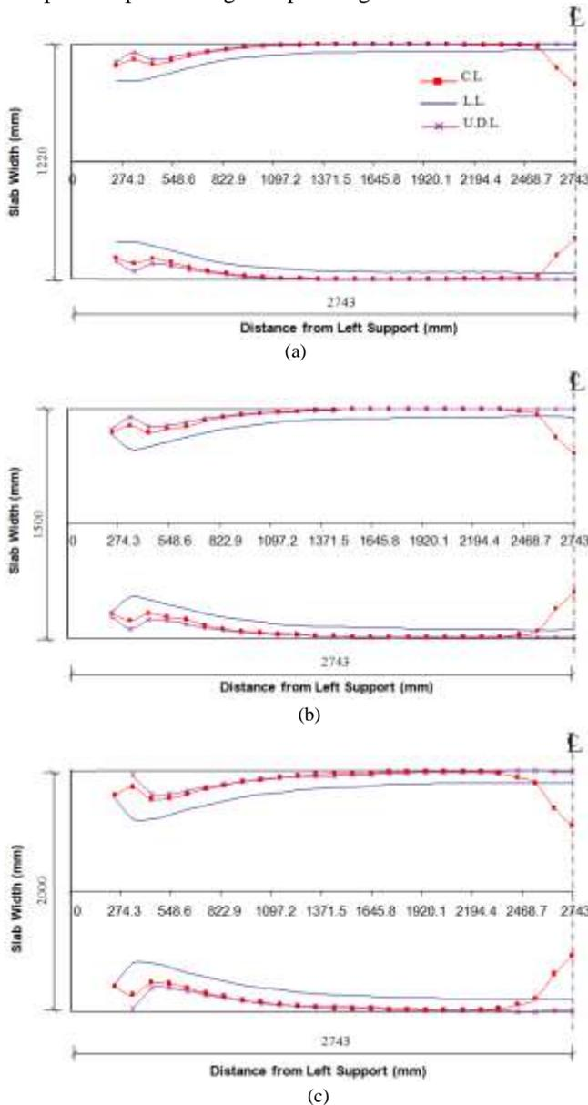
Fig. 6. Effective width for various loads, (a)  $b/L = 0.222$ , (b)  $b/L = 0.272$ , (c)  $b/L = 0.364$ .
