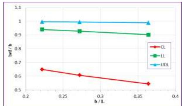
Fig. 5. Effect of panel proportion ( $b/L$ ) on the effective slab width ratio.
