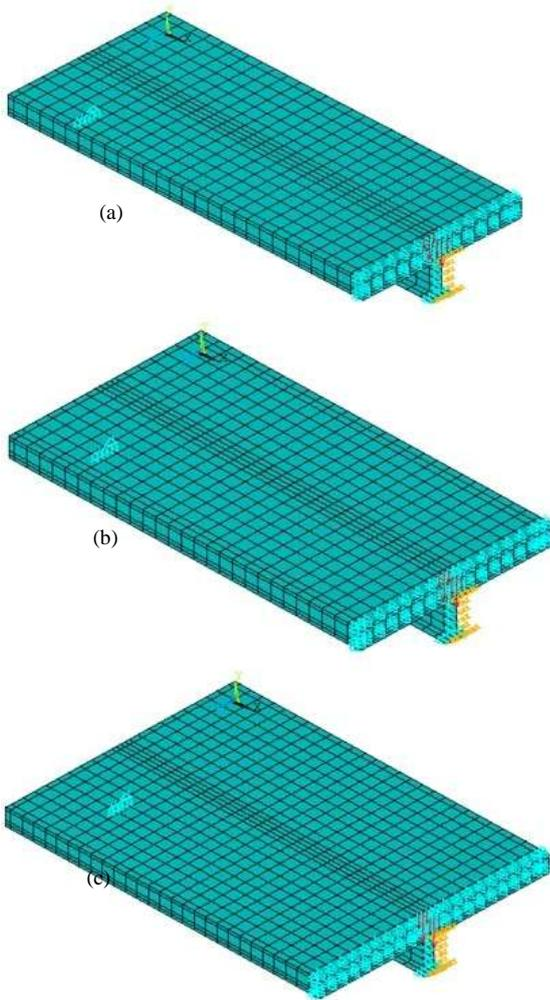
Fig. 4. Three dimensional finite element mesh for composite beam with different slab breadth, (a)  $b/L = 0.111$ , (b)  $b/L = 0.272$ , (c)  $b/L = 0.364$ .
