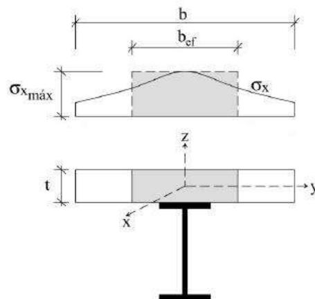
Fig. 2. Shear lag and effective width in a composite beam.
