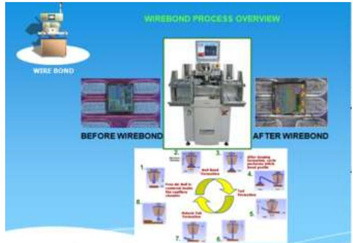
Fig. 3. Wire bonding process mechanism.
