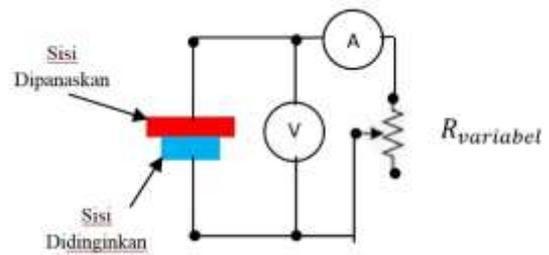
Fig. 8. Thermoelectric electrical testing circuit
