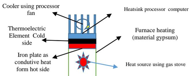
Fig. 6. Design of thermoelectric characteristics (furnace) test equipment
