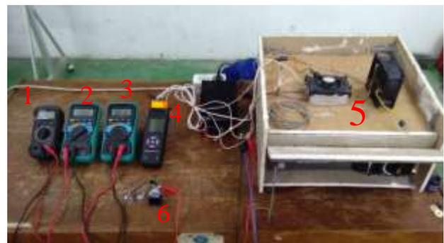
Fig. 9. Assembly thermoelectric electrical testing circuit
