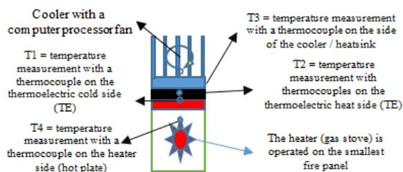
Fig. 7. Design of a thermoelectric characteristic test furnace
