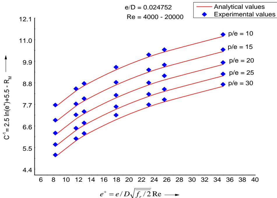
Fig.5 Comparison of  $C^{-1}$  for varying values of  $p/e$
