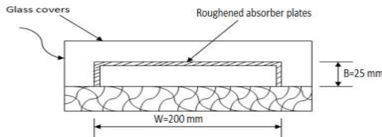
Fig. 1(b) Three sided roughened and one side smooth duct (present duct model)
