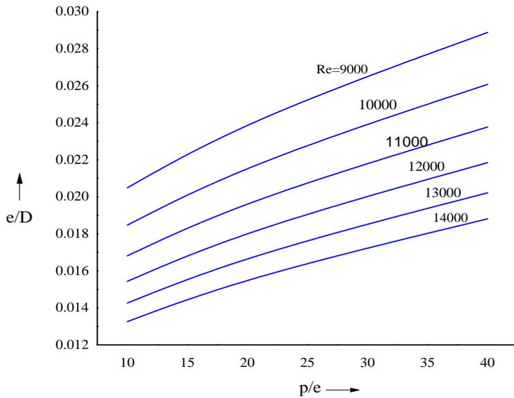
Fig.9.2 Optimal thermo hydraulic performance curve for three sides artificially roughened solar air heater
