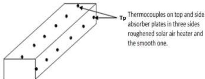
Fig. 3 (b) Thermocouple arrangement on top and sides of three sides roughened and smooth ducts
