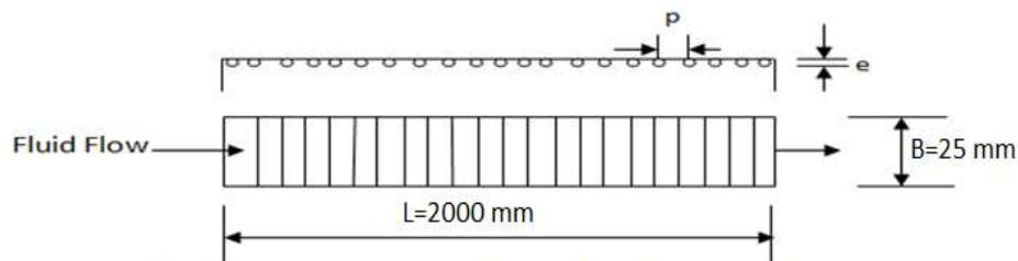
Fig. 2(b) Side absorber plate with artificial roughness
