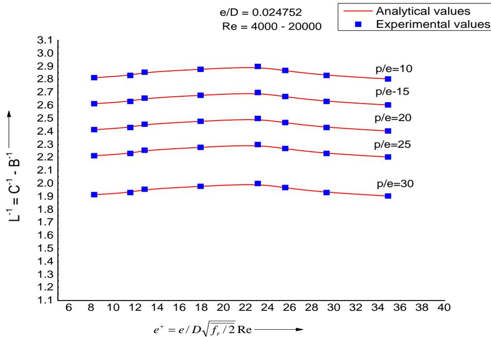
Fig.6 Comparison of efficiency parameter  $L^{-1}$  for varying values of  $p/e$
