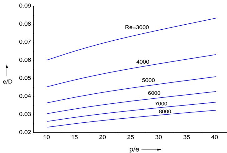
Fig.9.1 Optimal thermo hydraulic performance curve for three sides artificially roughened solar air heater
