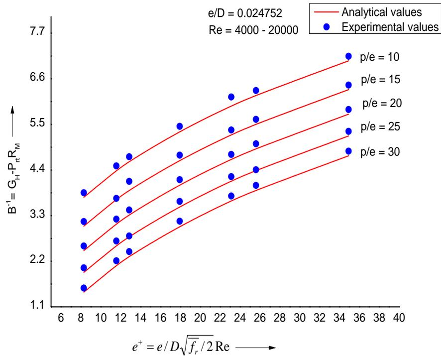
Fig.4 Comparison of  $B^{-1}$  for varying values of  $p/e$
