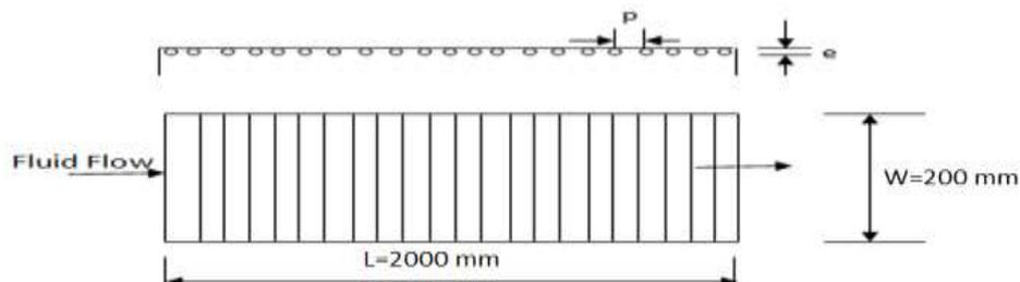
Fig. 2(a) Top absorber plate with artificial roughness
