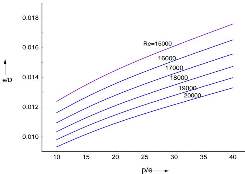
Fig.9.3 Optimal thermo hydraulic performance curve for three sides artificially roughened solar air heater
