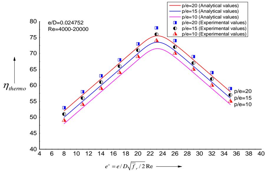
Fig.8 Efficiency versus Roughness Reynolds number
