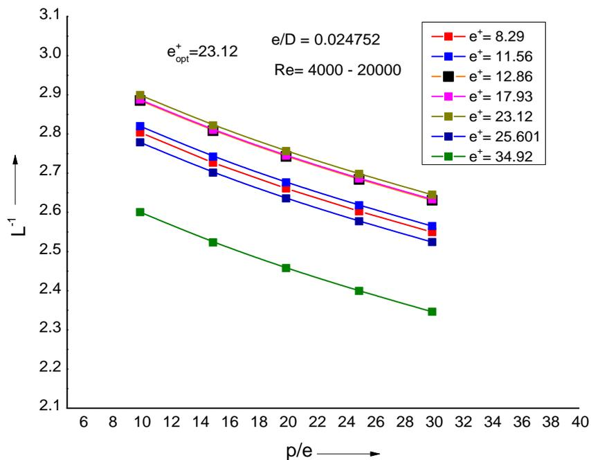
Fig.7 Efficiency parameter  $L^{-1}$  as a function of  $p/e$  and  $e^+$
