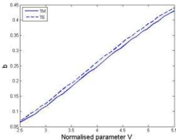
Fig. 2. The normalized modal index  $b$  as a function of  $V$  for fundamental TE and TM modes.
