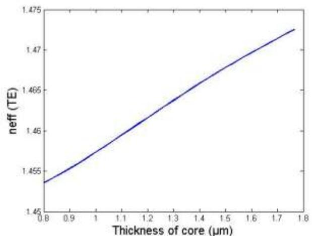
Fig. 4. effective refractive index as a function of thickness for fundamental TE mode
