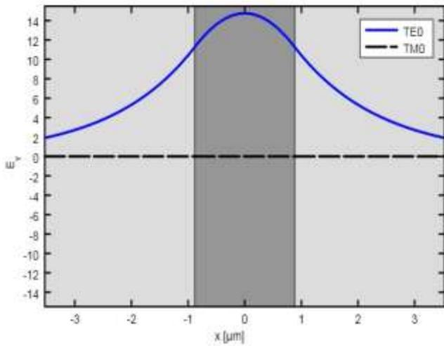
Fig. 5. the field distribution of the TE and TM fundamental modes for the wavelength 1.55 μm.
