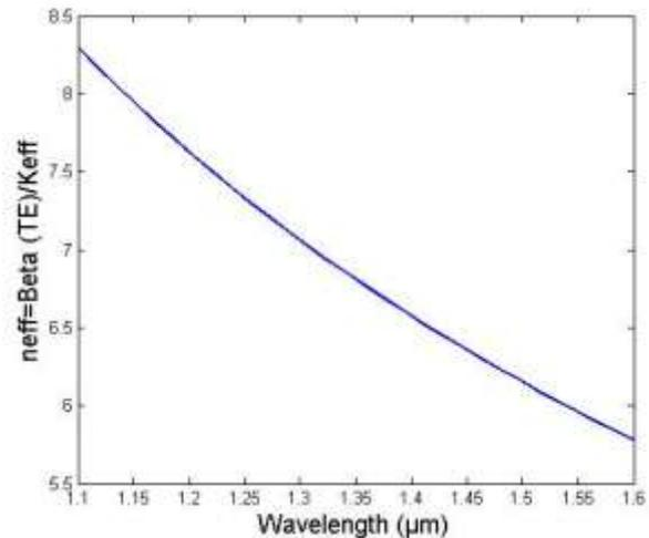
Fig. 3. effective refractive index as a function of wavelength for fundamental TE mode
