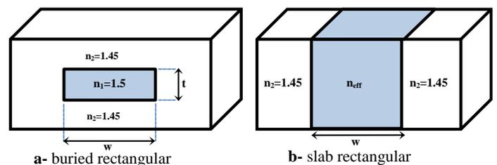
Fig. 1. The reduction of a- buried rectangular waveguide to b- slab waveguide by EIM
