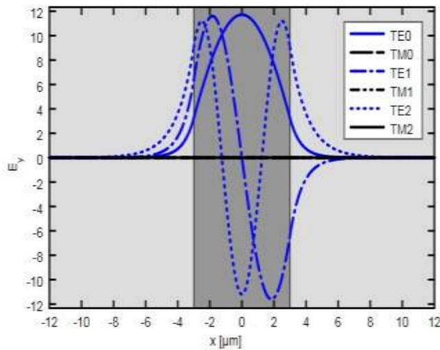
Fig. 6. the field distribution of the TE and TM higher order modes for the wavelength 1.55 μm.
