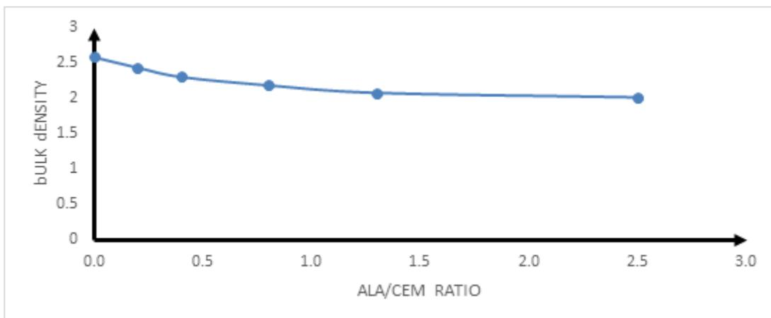
Fig. 3. Variation of Almond Leaf Ash / Cement Content (%) with Bulk Density (g/cm<sup>3</sup>)
