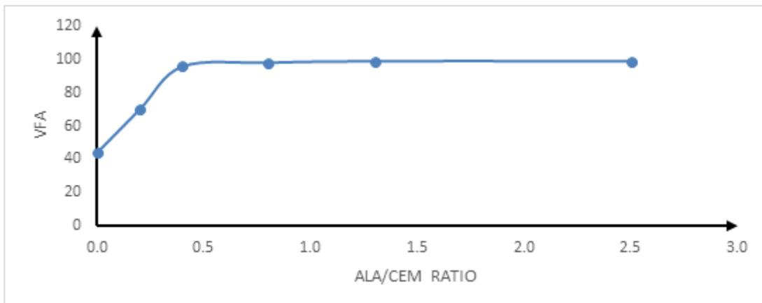
Fig. 6. Variation of Almond Leaf Ash Content (%) with Voids Fill in Aggregate (%)
