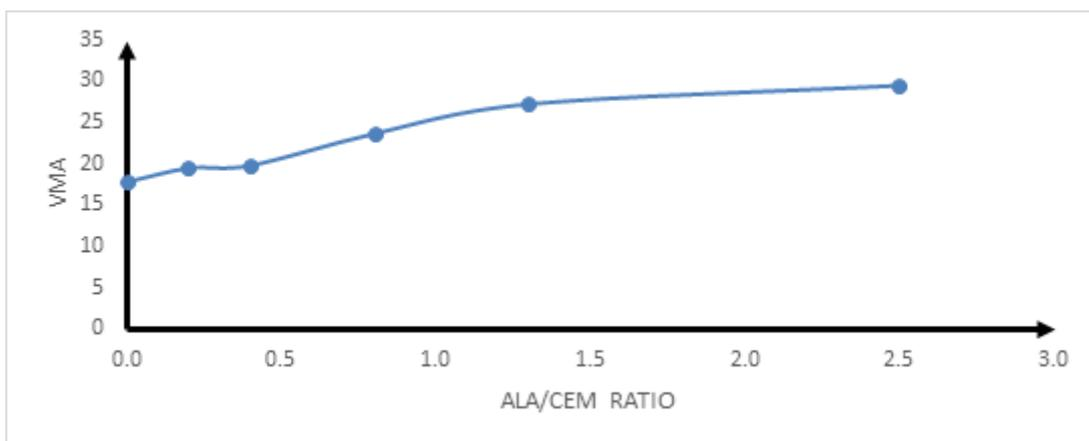
Fig. 5. Variation of Almond Leaf Ash /Cement Content (%) with Voids Mineral Aggregate (%)
