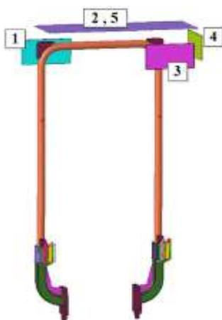
Fig. 2. ROPS loading sequence.
