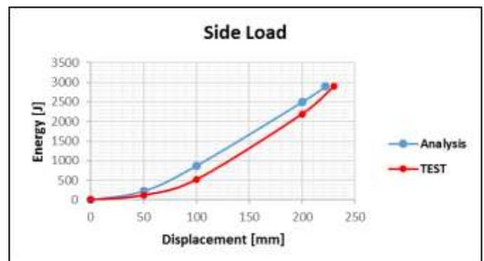
Fig. 7. Displacement – Energy curves obtained from analysis and test for side loading.
