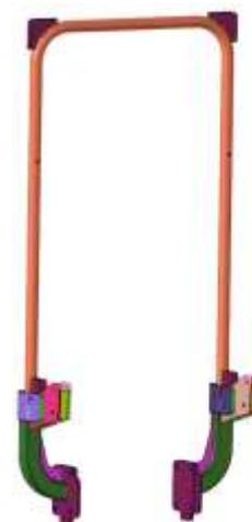
Fig. 4. Finite element model of the ROPS.
