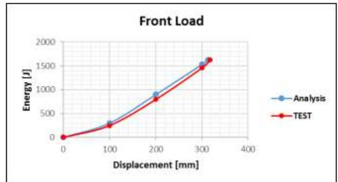
Fig. 6. Displacement – Energy curves obtained from analysis and test for front loading.
