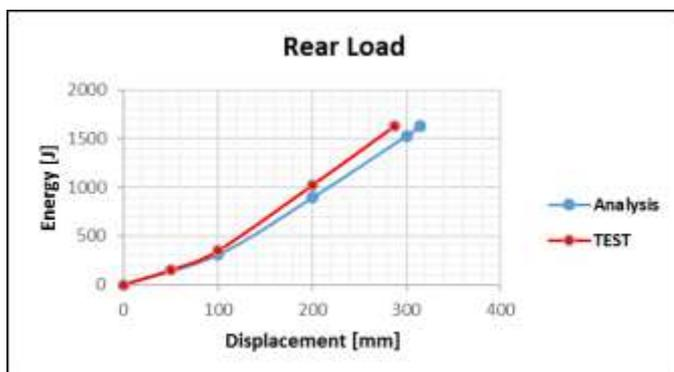
Fig. 5. Displacement – Energy curves obtained from analysis and test for rear loading.
