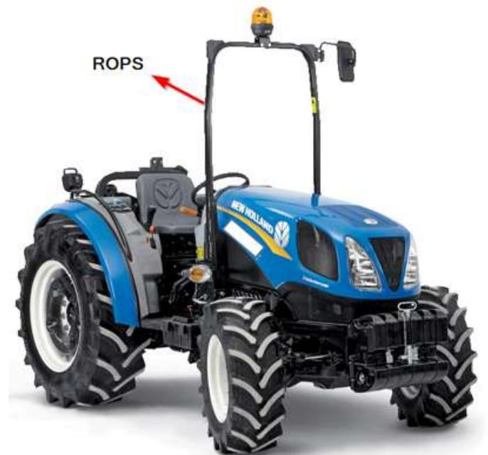
Fig. 1. Example of a frame type front ROPS.
