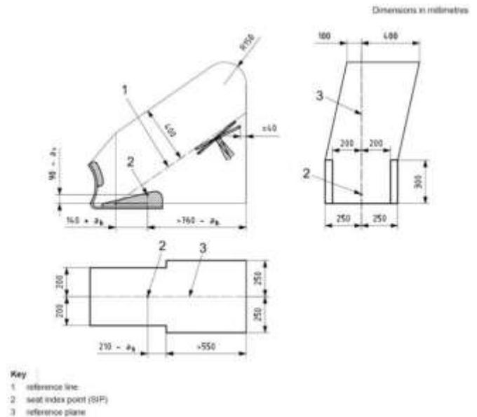
Fig. 3. Clearance zone calculation<sup>3</sup>.
