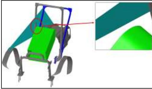
Fig. 8. Gap between clearance zone and ground plane.
