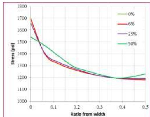
Fig. 10. Stress distribution (shear lag) in the top flange of the steel girder with two rectangular opens.
