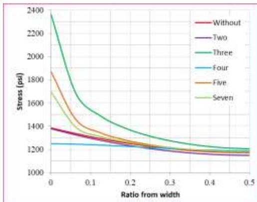
Fig. 3. Stress distribution (shear lag) in the top flange of the steel girder due to changing number of diaphragms.
