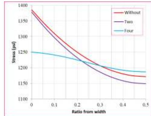
Fig. 4. Stress distribution (shear lag) in the top flange of the steel girder due to using 0, 2 and 4 diaphragms.
