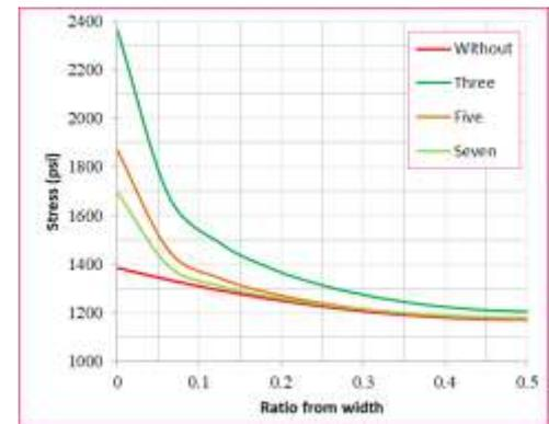
Fig. 5. Stress distribution (shear lag) in the top flange of the steel girder due to using 0, 3, 5 and 7 diaphragms.
