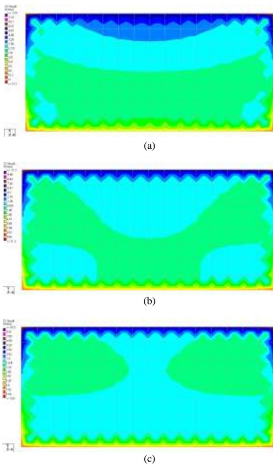
Fig. 8. Stress contours in the mid-span diaphragm of the steel girder, (a) with three diaphragms, (b) with five diaphragms (c) with seven diaphragms.
