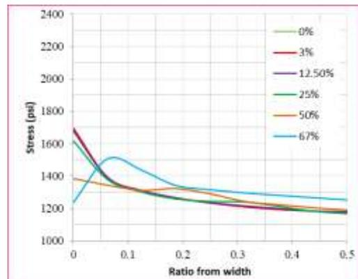
Fig. 9. Stress distribution (shear lag) in the top flange of the steel girder with single rectangular open.
