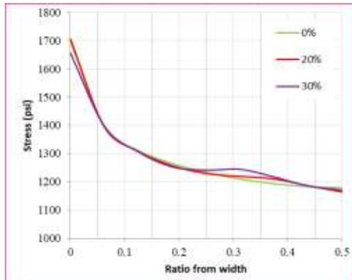
Fig. 11. Stress distribution (shear lag) in the top flange of the steel girder with diaphragms like cross.
