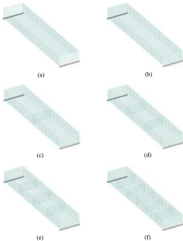
Fig. 2. Finite element modeling of the steel girder, (a) without diaphragms, (b) with two diaphragms, (c) with three diaphragms, (d) with four diaphragms, (e) with five diaphragms, (f) with seven diaphragms.
