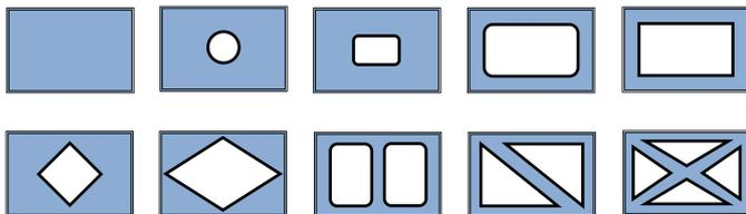
Fig. 1. Different types of steel diaphragms.
