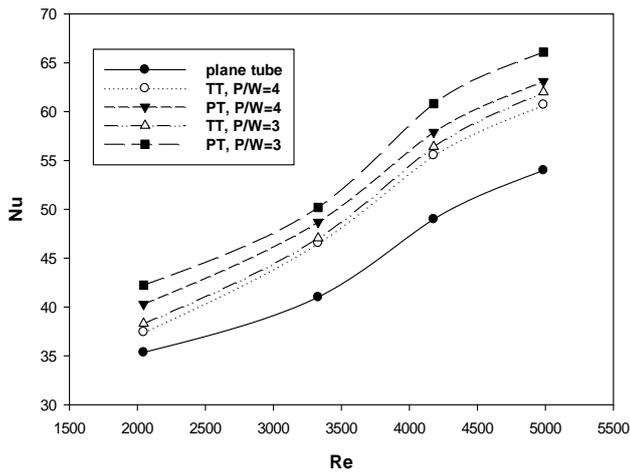
Fig. 10. Effect of twist ratio on Nusselt number.
