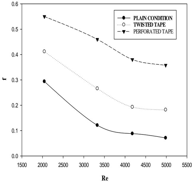
Fig. 7. Variation of friction factor for twist ratio 4.
