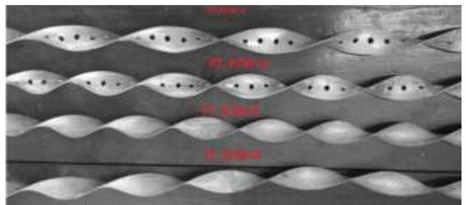
Fig. 5. Perforated and typically Twisted tapes.
