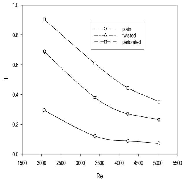
Fig. 6. Variation of friction factor for twist ratio 3.
