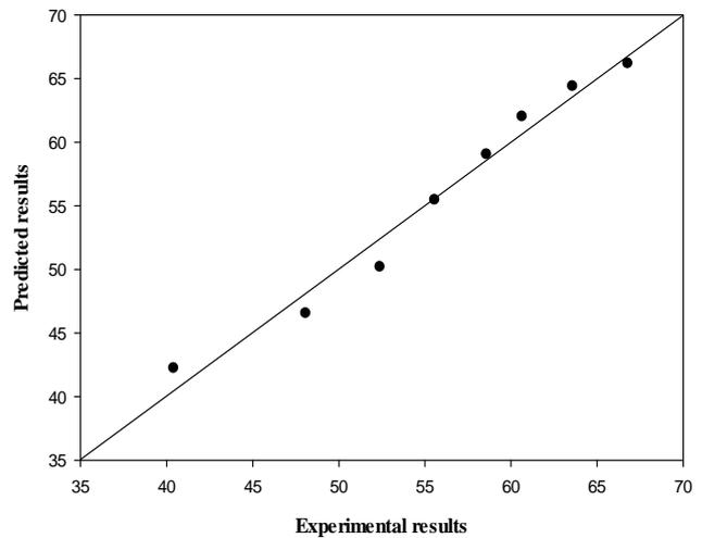
Fig. 12. Comparison between predicted and experimental Nusselt number.
