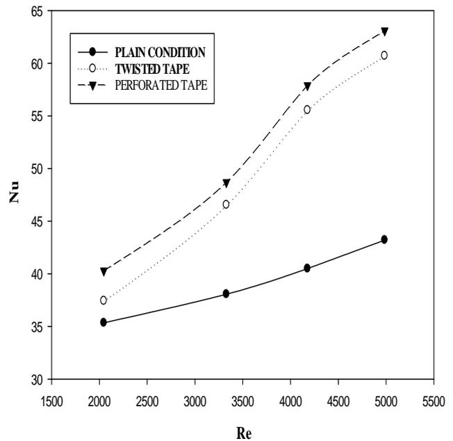
Fig. 9. Variation of Nusselt number with Reynolds number for twist ratio 4.
