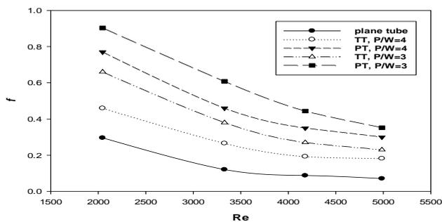
Fig. 11. Effect of twist ratio on Friction factor.
