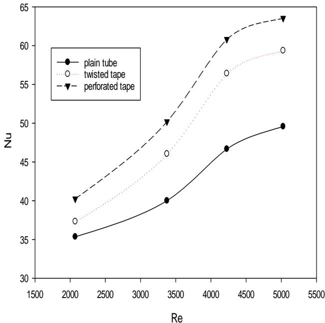
Fig. 8. Variation of Nusselt number with Reynolds number for twist ratio 3.
