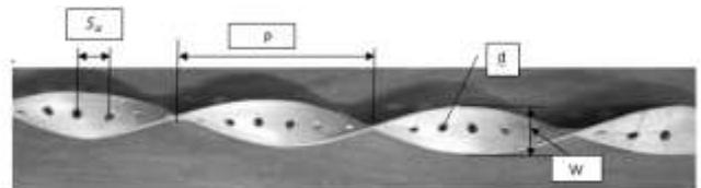
Fig. 4. Perforated twisted tape.
