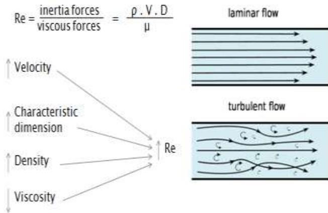
Fig. 1. Laminar and turbulent flow.
