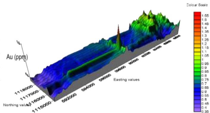
Fig. 6. 3d Surface map for Au using Kriging.
