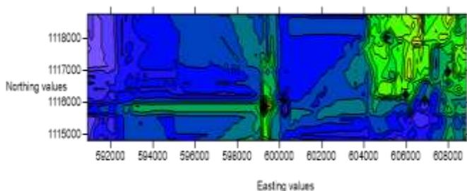
Fig. 5. Contour map for Au using Kriging.
