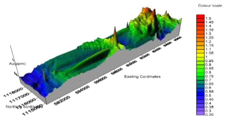
Fig. 8. 3d surface map for Au using IDW.
