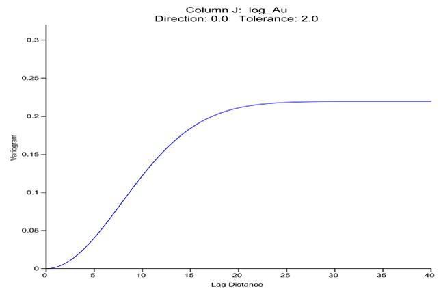
Fig. 4. Variogram plot for Au fitted with gaussian curve. From the Graph above, the following parameters were observed Nugget effect = 0, Range (a) = 20, Sill (C) = 0.23.
