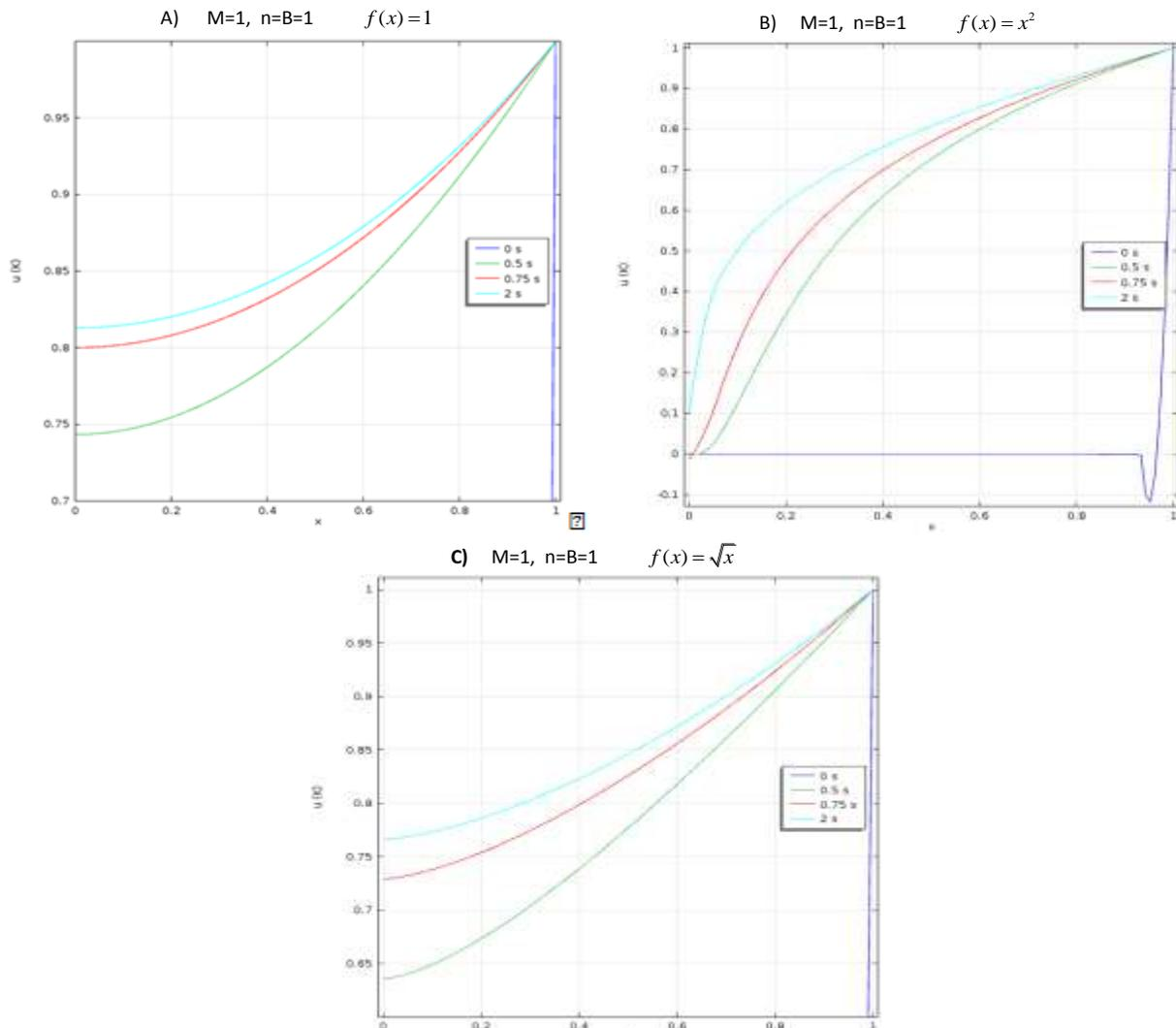
Fig. 2. The transient heat transfer of rectangular, parabolic, and convex profiles. (A: rectangular, B: Parabolic and C: convex profiles).
