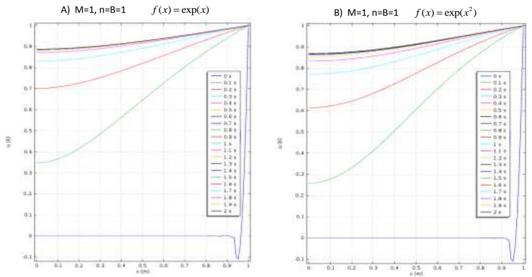
Figure 4. The transient heat transfer for exponential profiles.
