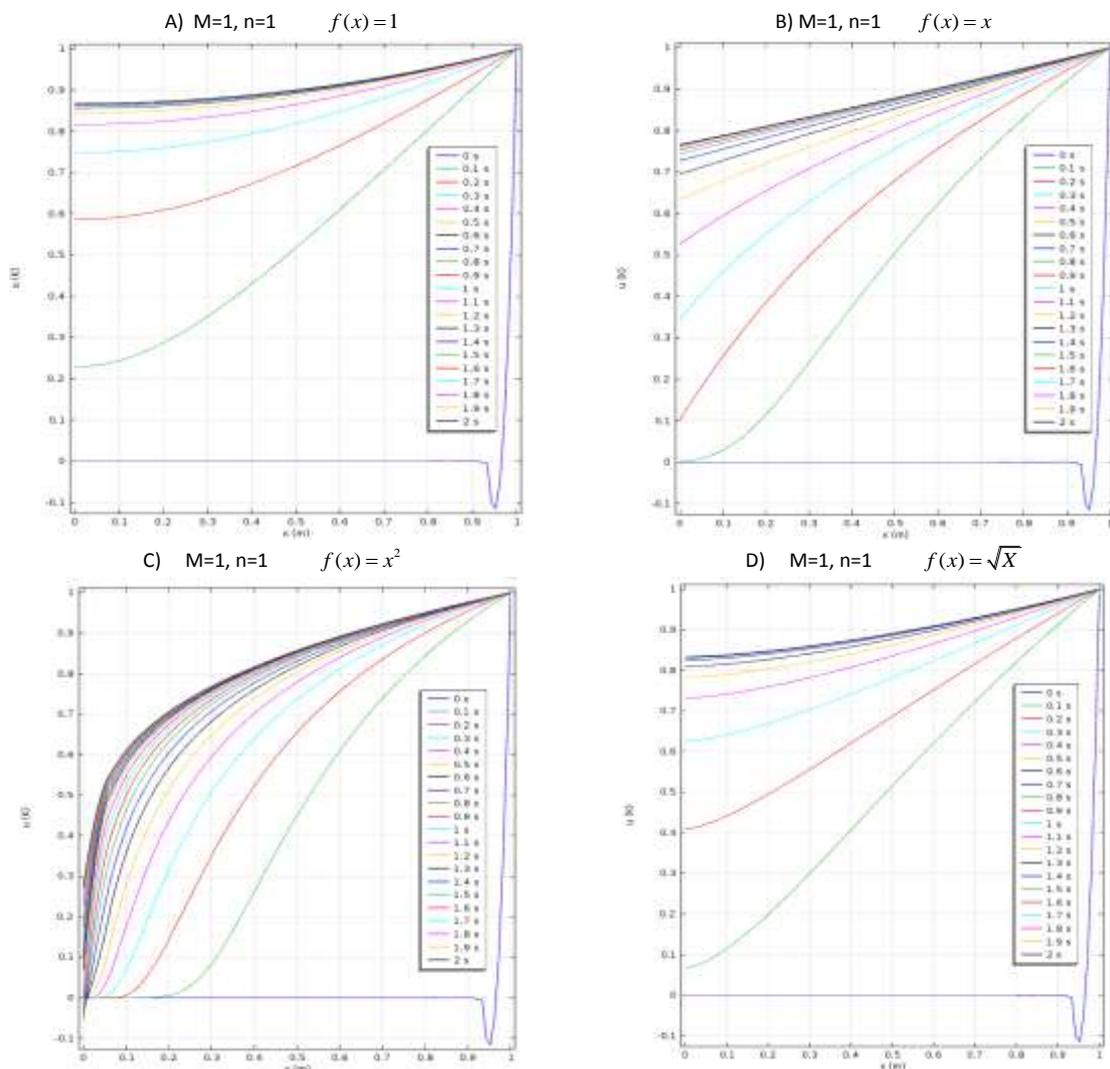
Figure 5. The transient heat transfer of rectangular, triangular, parabolic and convex profiles using Kadar et al. [26] PDE and considering a nonlinear thermal conductivity.
