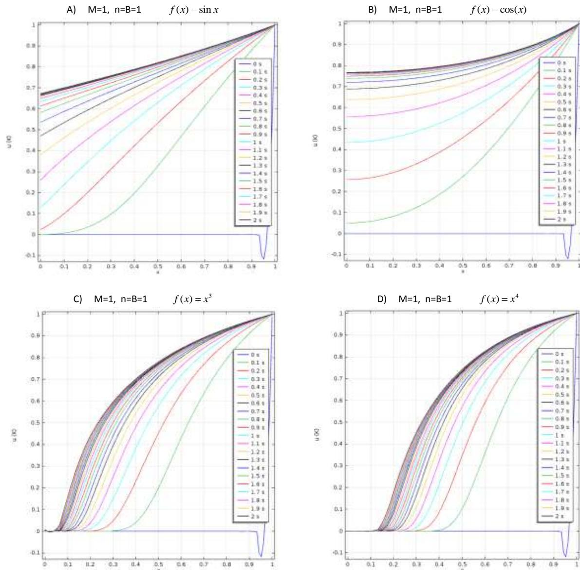
Fig. 3. The Transient heat transfer for sinusoidal, cosine, third order and fourth order profiles. (A: sinusoidal, B: Cosine, C: third order and D: forth order profiles).
