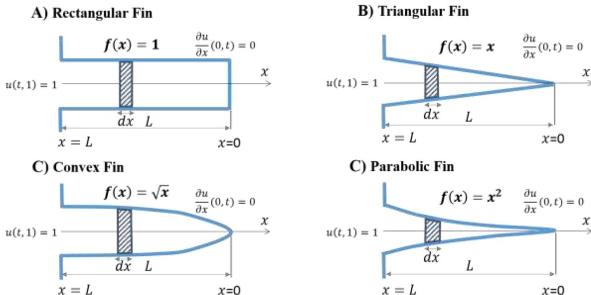
Fig. 1. Four different profiles of fins including rectangular, parabolic, convex, exponential, sinusoidal, and cosine profile.
