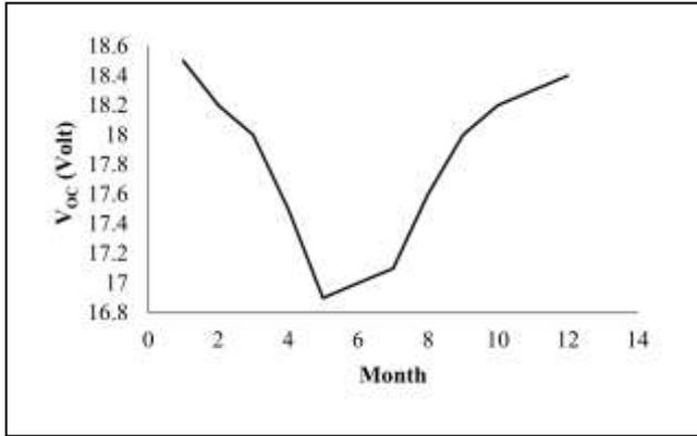
Fig. 1. The open circuit voltage distribution through the year.
