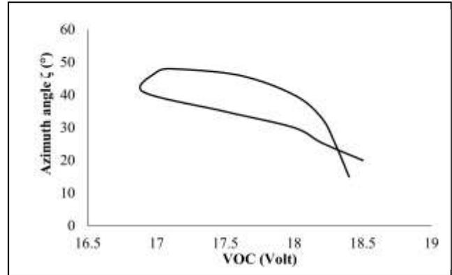
Fig. 3. The azimuth angle relation with open circuit voltage.
