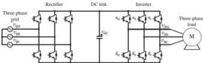
Fig. 3. Source connected with IGBT rectifier for AC-DC-AC conversion.
