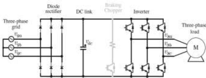
Fig. 2. Source connected with diode rectifier for AC-DC-AC conversion.
