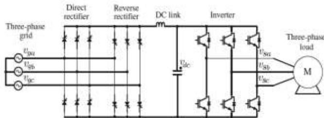
Fig. 4. Source connected with thyristor rectifier for AC-DC-AC conversion.
