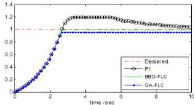
Fig. 17. Step response OF load in different controllers, GA-FLC and BBO-FLC and PI controller.
