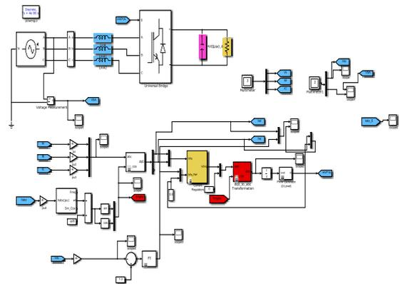
Fig. 6. The simulation model for three phase PWM rectifier with PI control.
