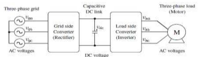
Fig. 1. Source connected machine by power electronic converter.
