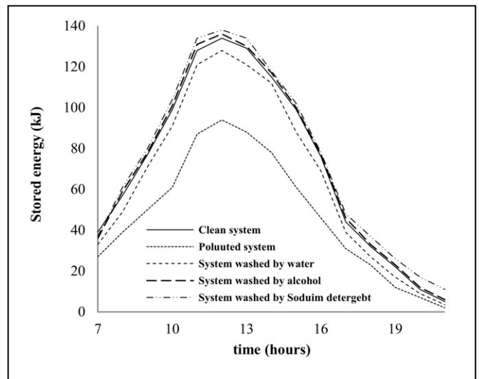
Fig. 4. The stored energy in the target for the studied cases distributed with time
