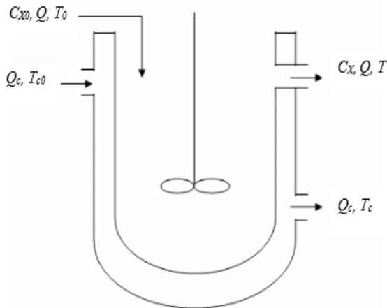
Fig. 1. A typical diagram of a continuous stirred tank reactor.
