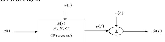
Fig. 3. Linear continuous-time process with input and output noise.
