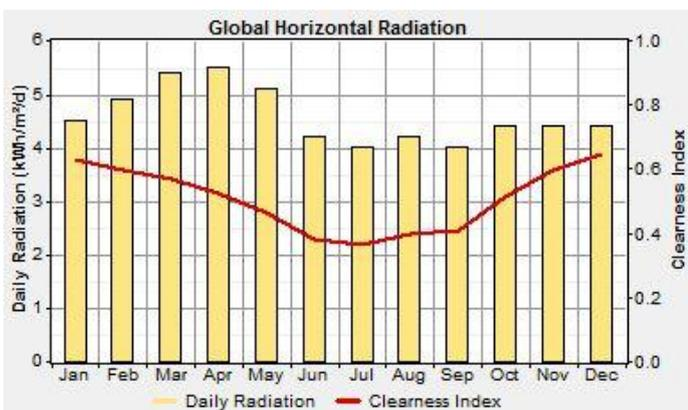
Fig. 3. Graphical representation of daily solar radiation in HOMER.
