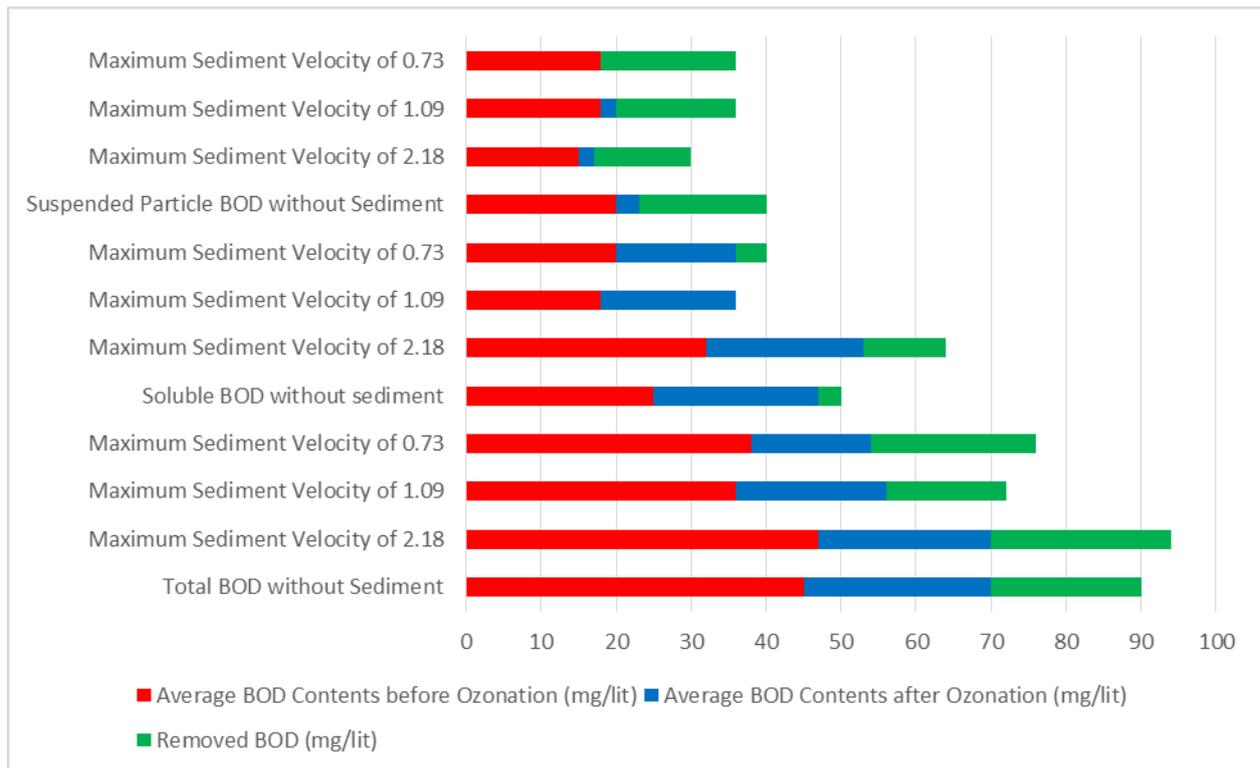
Fig. 1. Average wastewater's BOD removing before and after ozonation.
