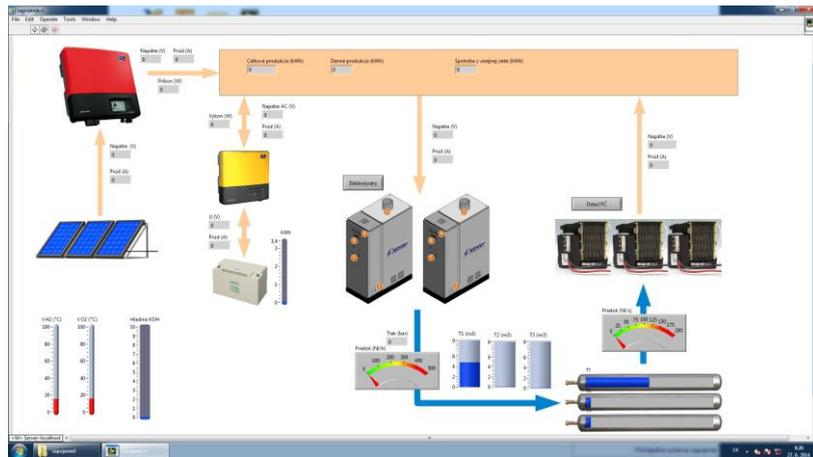
Fig. 11. Hydrogen accumulation system visualization.
