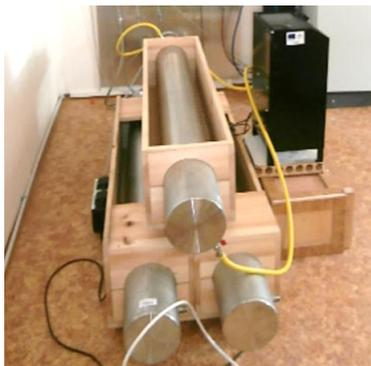
Fig. 7. HBond©9000 metal hydride vessels.
