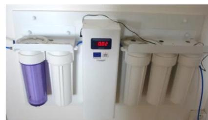
Fig. 5. SolPure water deionizer.
