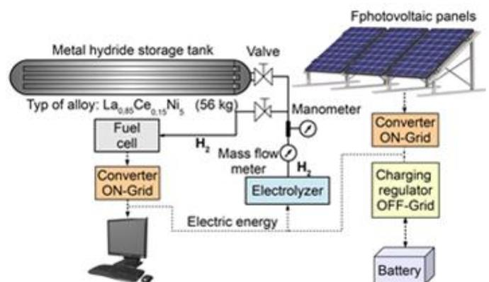
Fig. 1. The solar energy accumulation system using hydrogen technology.
