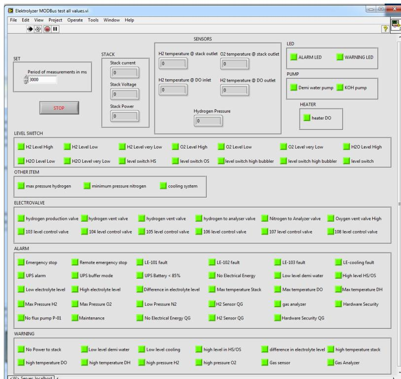
Fig. 12. Visualization of hydrogen accumulation system in the environment of LabView for electrolyzer.
