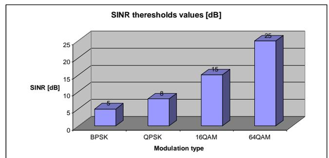
Fig. 2. Minimal SINR values in 802.11 standards.
