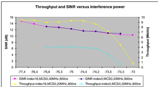
Fig. 10. Throughput and SINR versus interference power level for the following attributes: simulationTime=2s, BPSK, Friis loss model, distance=50 m, Rx=-62,6 dBm.
