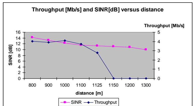
Fig. 8. Throughput and SINR versus distance for the following attributes: simulationTime=2s, index=0 (MCS=0, BPSK, 20MHz channel width, 800ns guard interval), Friis loss model. waveformPower=0.00001W.
