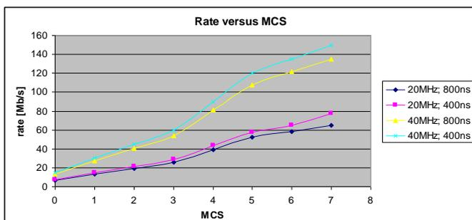
Fig. 1. Maximal theoretical transmission rate in 802.11n standard for following parameters: guard interval 400/800 ns, channel width 20/40 MHz and modulation type BPSK (MCS=0), QPSK (MCS=1;2), 16 QAM (MCS=3;4) i 64 QAM (MCS=5;6;7).
