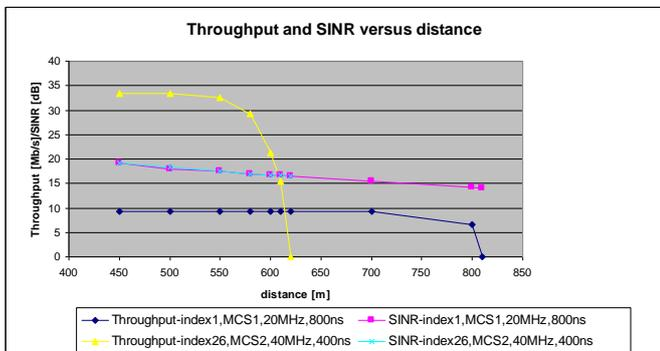
Fig. 11. Throughput and SINR versus interference power level for the following attributes: simulationTime=2s, QPSK, Friis loss model, waveformPower=0.00001W.
