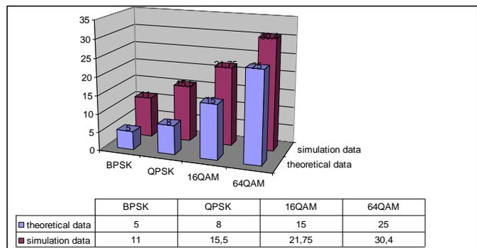
Fig. 14. Comparison of theoretical and simulation data of SINR values.
