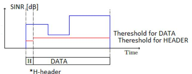
Fig. 4. Comparison of theoretical SINR requirements with the Real SINR value during the packet transmission.
