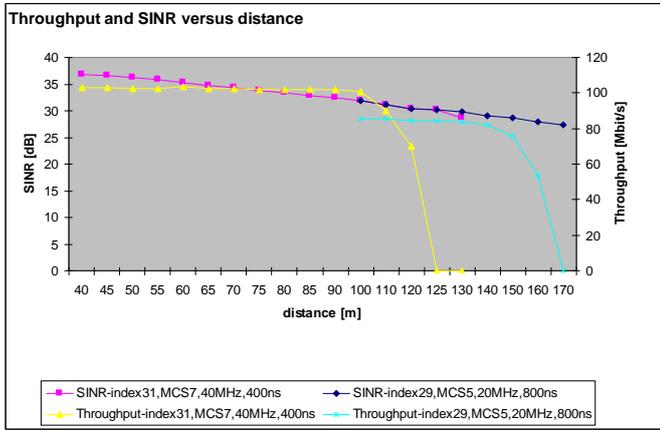
Fig. 9. Throughput and SINR versus distance for the following attributes: simulationTime=2s, 64QAM, Friis loss model, waveformPower=0.00001W.
