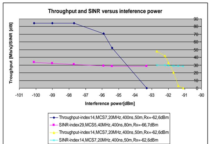
Fig.13 Throughput and SINR versus interference power level for the following attributes: simulationTime=2s, 64QAM, Friis loss model
