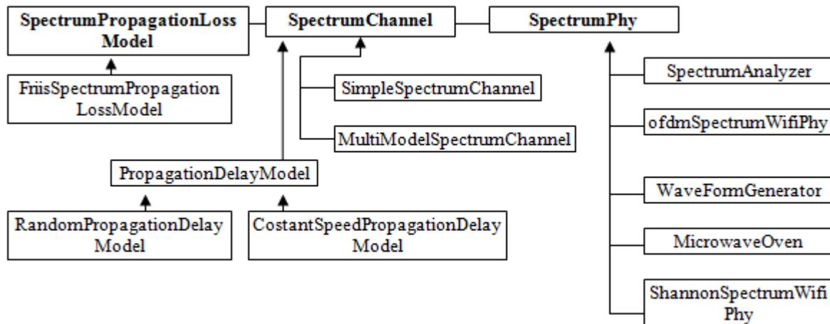
Fig. 3. UNL diagram of PHY layer of radio channel.
