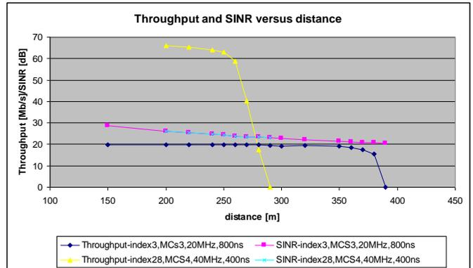
Fig. 12. Throughput and SINR versus interference power level for the following attributes: simulationTime=2s, 16QAM, Friis loss model, waveformPower=0.00001W.
