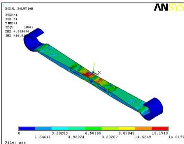
Fig. 1.7. Equivalent stress of steel leaf spring.
