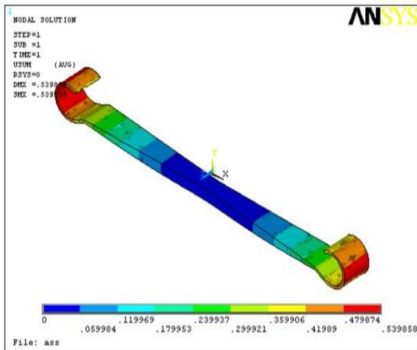
Fig. 1.6. Total Deformation of steel leaf spring.
