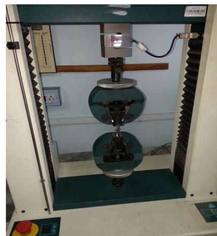
Fig. 3. Universal testing machine.
