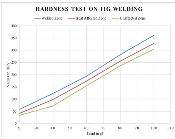
Fig. 8. Hardness testing graph.
