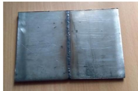
Fig. 2. TIG welded specimen.
