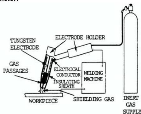
Fig. 1. TIG welding machine setup.
