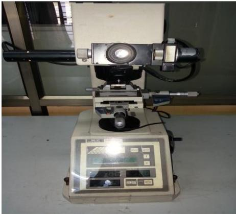
Fig. 6. Vickers hardness test machine.
