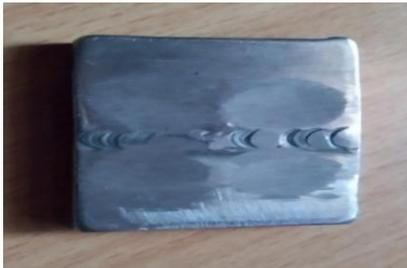
Fig. 7. Hardness test specimen.
