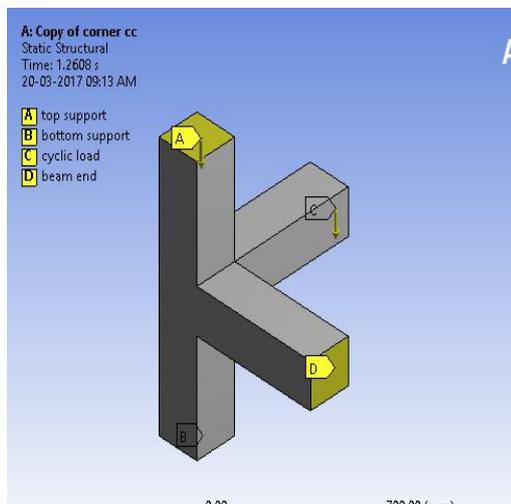
Fig. 4. Support conditions for corner beam column joint.
