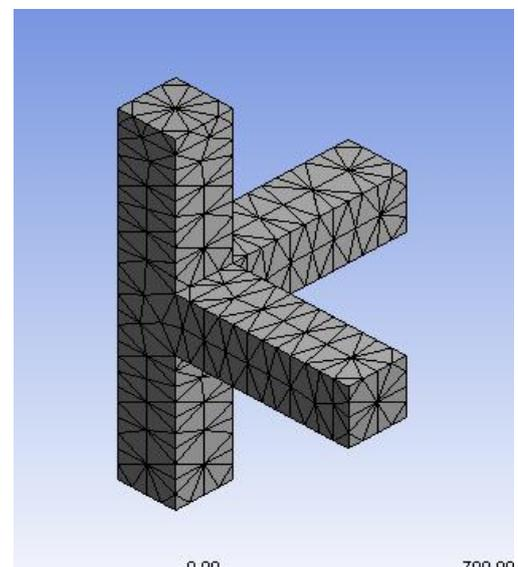
Fig. 3. Meshing diagram.
