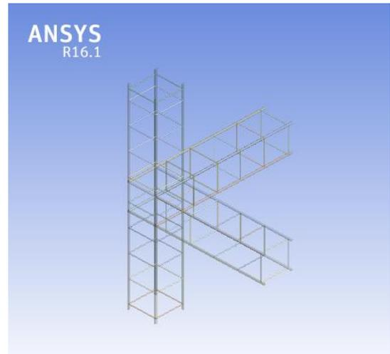
Fig. 1. Reinforcement model having conventional stirrups.
