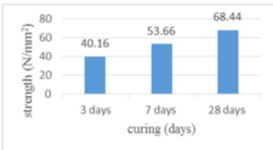
Fig. 1. Graphical representation of compressive strength of control mix.
