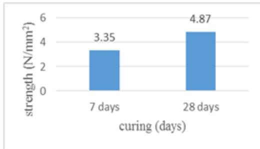
Fig. 5. Graphical representation of split tensile strength of optimum percentage of metakaolin.
