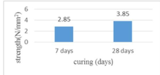
Fig. 2. Graphical representation of split tensile strength of control mix.
