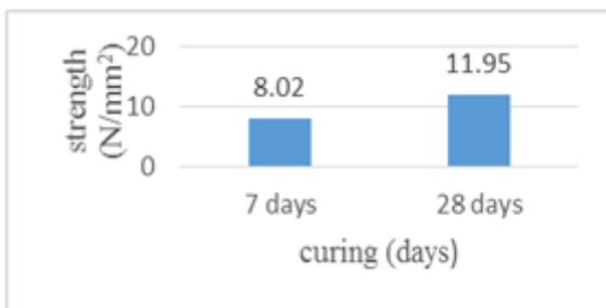
Fig. 6. Graphical representation of flexural strength of optimum percentage of metakaolin.
