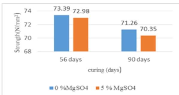
Fig. 7. Graphical representation of specimen exposed to magnesium sulphate solution.
