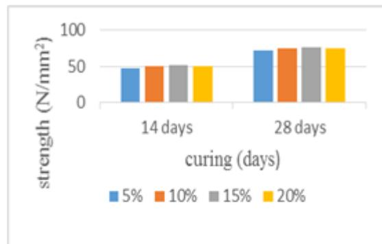
Fig. 4. Graphical representation of compressive strength of various percentage of metakaolin.
