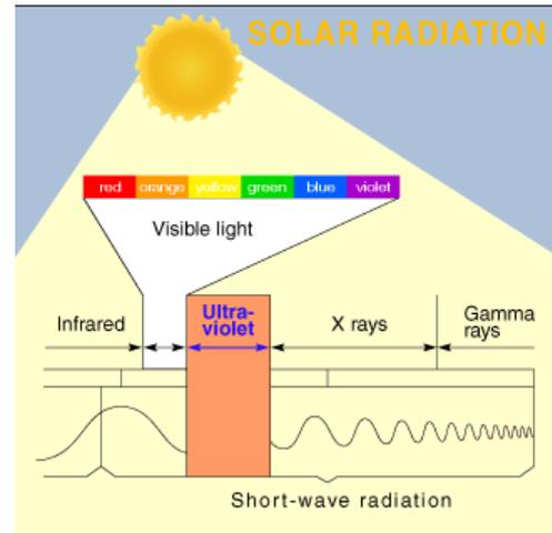
Fig. 2.1. Spectrum of electromagnetic waves.
