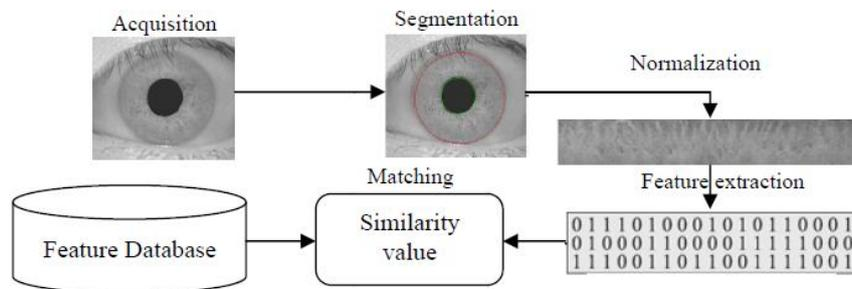
Fig 1.1. A typical iris recognition system.
