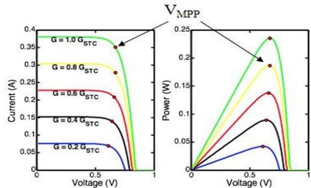
Fig. 2. PV cell voltages versus the load current and the power consumption on the target device, and solar irradiance.
